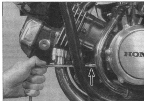
**8.10 Inlet water pipe clamp bolt location (arrow)**
