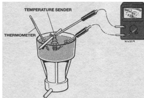
4.7 Cooling fan thermostatic switch test set-up
